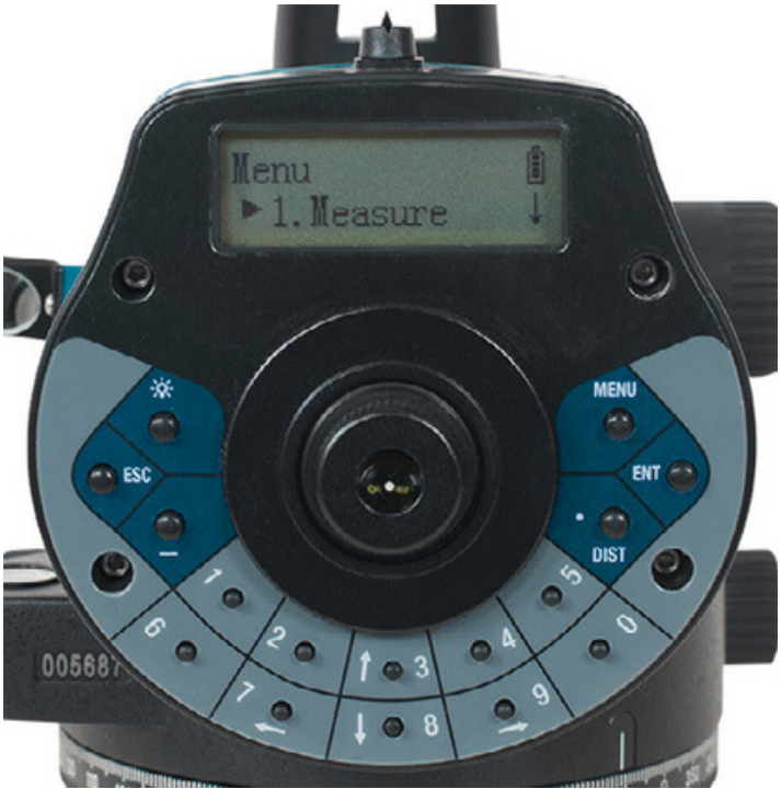
Figure 3.1 Control and display unit of the DLS-15 digital level
